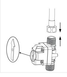
installed on the water supply line before the solenoid valve to be able to turn off the water supply in case of damage or servicing of the system.
