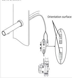
8. 6VDC adapter is connected to red-brown cable pair.
